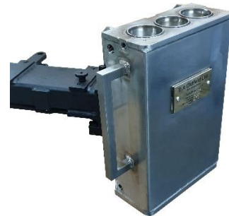
Figure 3. shows a funnel box on a DAO ALS quick change mounting arm.
