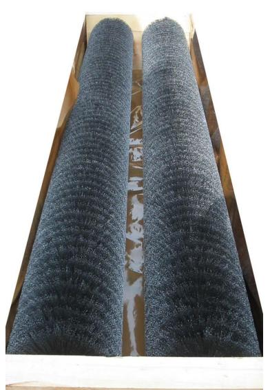
The primary purpose of the lehr belt cleaning rollers is to clean all the small glass particles and burnt grease off the lehr belt to prevent the particles coming in contact with the new formed glass container bases, this takes place at the cold end of the lehr.
