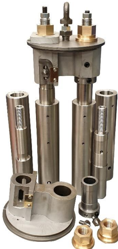
Figure 2. Shows a traditional Plunger Chuck created new from original drawings
