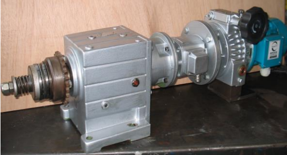
Figure 3. Stacker drive unit with clutch break & motor.
