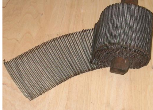
Figure 8. Woven wire belt.
