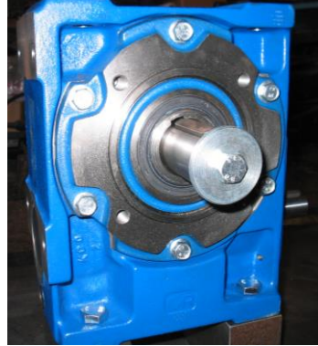
Figure 2. Rossi 16:1 ratio gear box.
