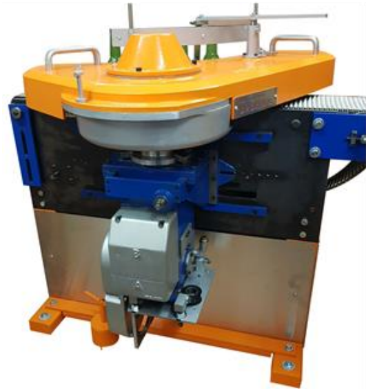
Figure 2. Inverted belt conveyor end with moving gear box and 700 transfer fitted.
