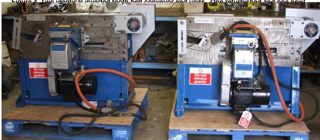
Figure 4. Two identical inverted tooth belt conveyor end units. One refurbished and one new
