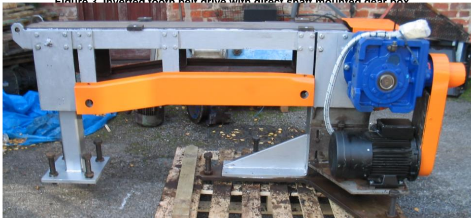
Figure 4. Two identical inverted tooth belt conveyor end units. One refurbished and one new
