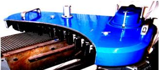
Our **A**dvanced **T**ransfer model 4000 is better known for it's handling of small ware at high speeds typically produced on triple or quad gob IS machines. D A Oldfield Ltd built on the success of this design by producing longer fingers and retracting cam to handle bottles up to 85mm diameter. The transfer unit is compact, simple to set up and job change due to "drop on" fingers quick-change cam and chain assembly.
