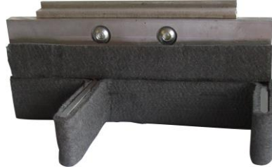
Figure 2. Pusher with high temp cloth insulation
