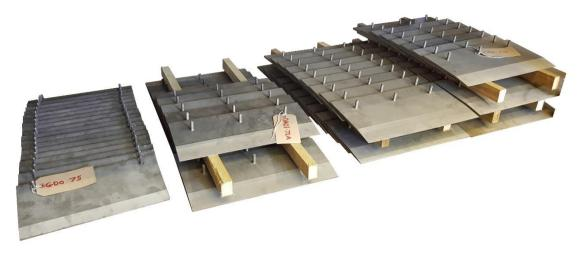
The purpose of the Lehr Dead Plates is to provide a stable flat platform for the bottle to be pushed between the Cross Conveyor and the Lehr Belt.
