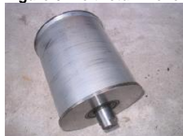
Figure 6. Belt return roller
