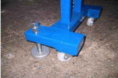
Figure 1. Conveyor legs showing jack screw and castors.
